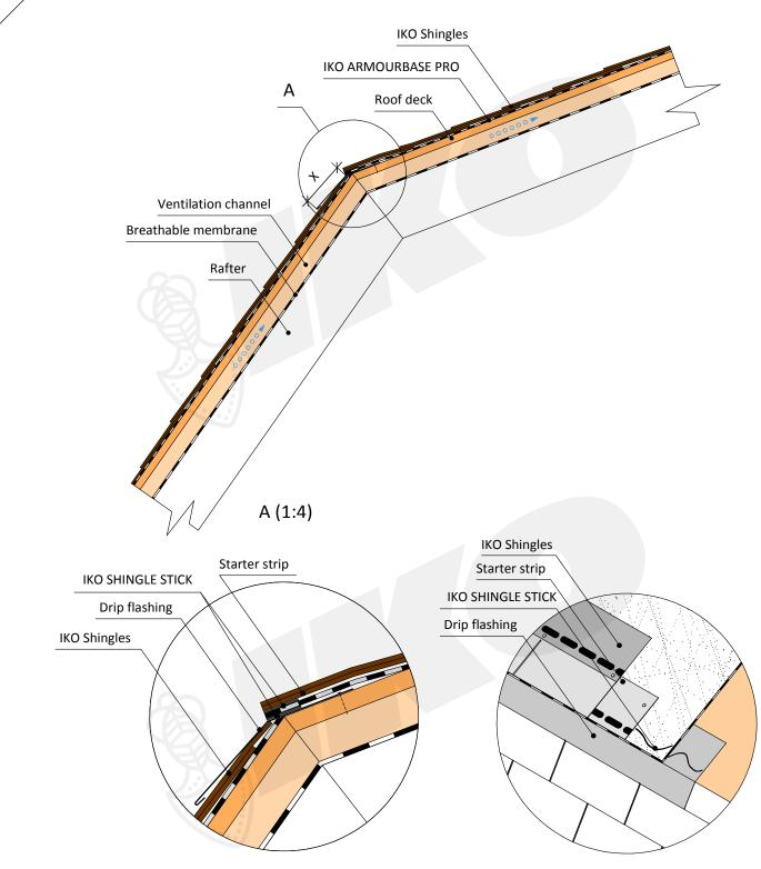
X - min 120, should be enlarge with a decreasing angle of a slope and/or requirements of local codes
