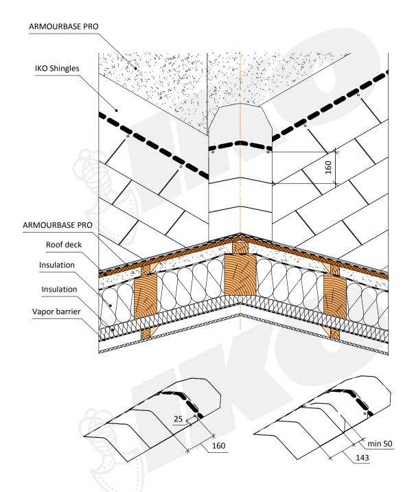
Apply the hip and ridge shingles double thickness by stacking two pieces and bending them over the hip or the ridge. Always ensure that, when installing the ridge covering shingle tabs, the nails of the upper shingle course (on both sides of the ridge) are covered.
